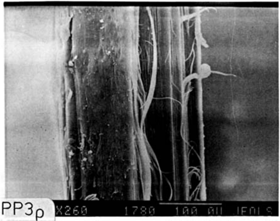
Figure 2 (a) Phase-contrast micrographs of the sections of the composites and (b) SEM micrographs of the corresponding fractures.
